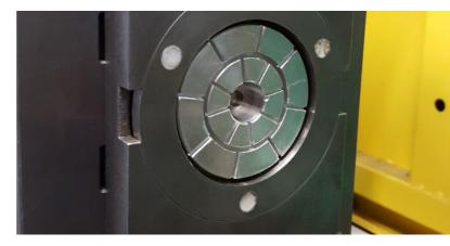
Figure 2: Tool cavity with core setter
